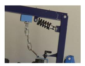
• The trolley has a reception base for the OAKBOT which makes it possible to maintain the OAKBOT in a fixed (non-suspended) position on the trolley. To fix the OAKBOT to the trolley using this device, firstly position the bottom of the OAKBOT in the reception base then rotate the OAKBOT until the holding mechanism snaps into place in the dedicated hole situated on the OAKBOT suspension hook.
