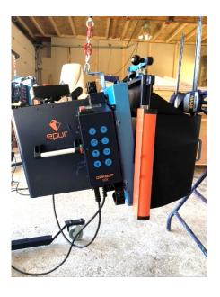
2. Once the bottom has been slotted in, redress the OAKBOT and lock in position using the 2 dedicated locking levers. Check that the lever goes to the end of its travel.
