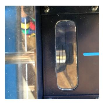
8. Then go to Y to align the top of the tool with the bottom of table Y. Come into slight contact with the table, being careful not to force. Once in contact, do not touch this axis any more until the calibration process is over.
