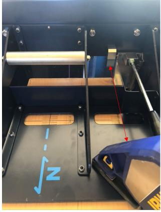
The lower surface of the table will be in contact with the surface of the workpiece, representing the reference along (Y).
