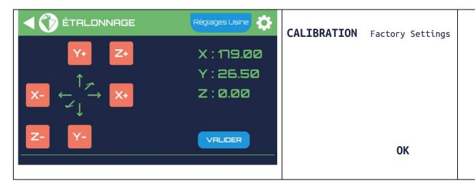
7. Initially, press Z+ until the end of the tool is aligned with the reference line on the polycarbonate clamping plate. Once aligned, do not touch this axis any more until the calibration process is over.
