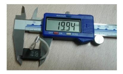
They will need to be replaced if the measurement of what is left is less than 10mm.
