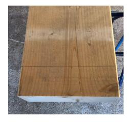
Trace a line parallel to the shoulder line (distance indicated by the machine depending on the type of tool)
