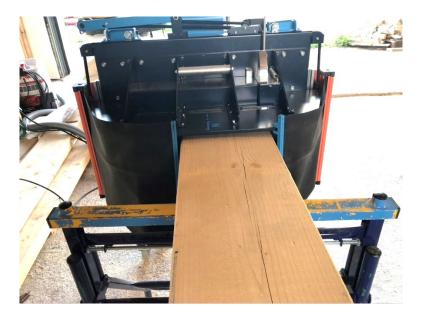
When carrying out edge machining with a piece that protrudes either side of the machine, putting this system in place is not necessary. In all other machining configurations, using this system is needed.
