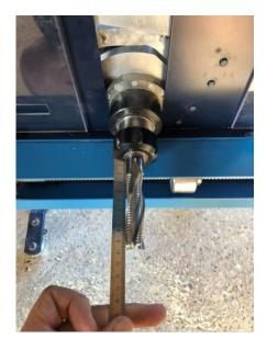
Incorrect measurement will cause machining that is non-compliant with the dimensional specifications you entered.
