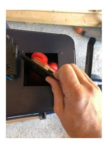
Unscrew the four assembly screws of the spindle motor switch casing.
