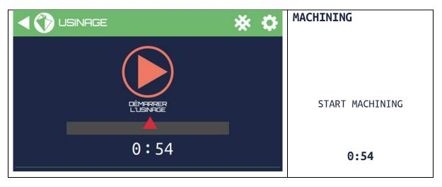
2. A warning window appears to confirm that the machine is properly positioned on the clamping unit. Once validated, if the reset button has not been engaged, the programme also requests you to reset the machine. You can now validate machining start-up. If you wish to cancel, press the cross located at the top right of the window. Otherwise, if you are sure you want to start machining, actuate the milling cutter and start the machine moving, press START MACHINING.
